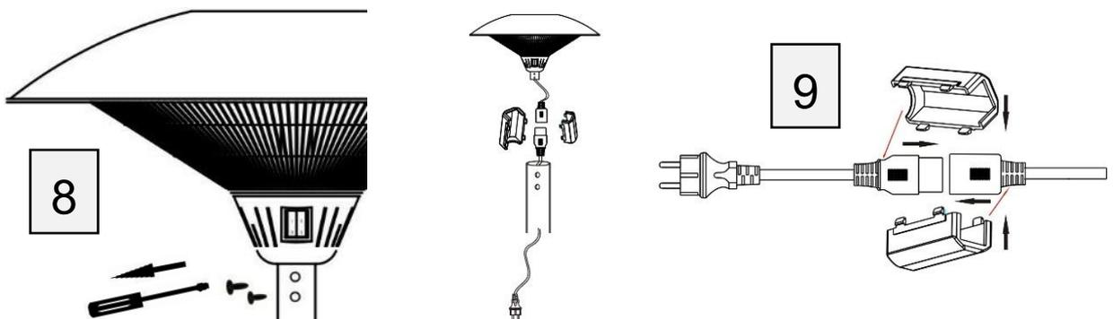
**Step 5:** Insert the heating head onto the pipe and screw in the screws again.
